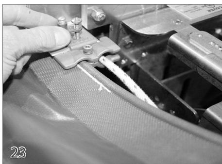
Use a 5/32" allen wrench to loosen the screw on top of the guide feed. Place the guide feed over the end of the track with the cover coming through one side and the rope through the other. Place a bonding lug (25) on a 10-32 X 1 3/4" screw (42) and insert the screw through the hole on top of the guide feed.
