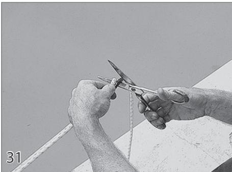
While pulling both ropes tight, use a lighter or torch to burn the rope in the location it will be cut. This will help them not fray after they have been cut. Cut the ropes so they are at least 8 ft long. In some cases you may only need to cut one rope. Use the lighter to reburn the cut ends of the rope if needed.
