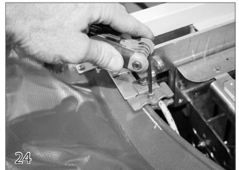
Use the allen wrench to tighten the screw that connects the two sections of guide feed together.
