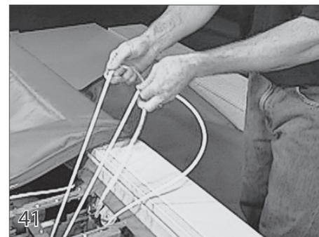
If both ropes are the same length, and the cover doesn't close squarely, shorten the rope for the side of the cover that doesn't close all the way. The amount that the rope is shortened is equal to the distance that the cover needed to travel to close all the way. After shortening the rope, run the switch in the cover position while holding the ropes.
