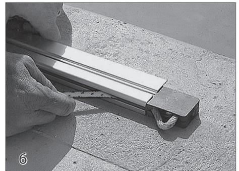
Feed the rope through the pulley (15) assembly. Insert the pulley with the rope onto the end of the track.
