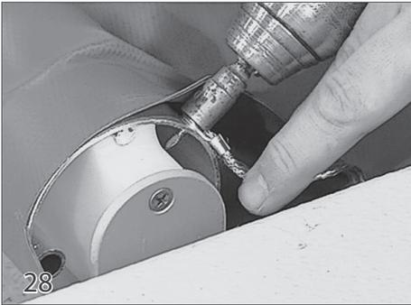
Connect the bonding wire that is attached to the front corner of the cover to the leading edge bar using a 10 x 1/2" tek screw (31). Be sure the screw doesn't interfere with the leading edge insert from moving freely inside the tube. Do this on both sides of the cover.
