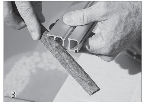
Before splicing the sections of track together, file all track ends thoroughly, rounding all edges and removing all burrs. Clean metal shavings from the track. This step is extremely important! If the track isn't filed smooth, damage can occur to the ropes, slider and cover.
