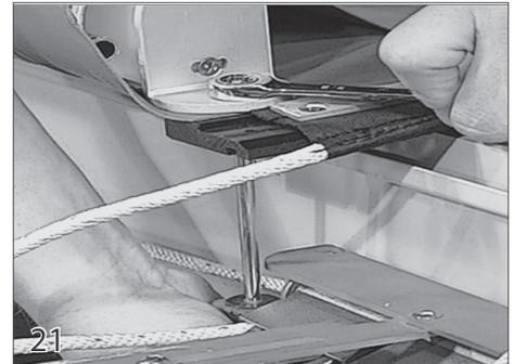
Secure the leading edge insert support bracket to the slider by placing the 10-32 X 1" screw up through the slider, through the hole in the front corner of the cover, and through the support bracket. Tighten completely using 10-32 nylock nut, then back the nut off 1/2 turn.
