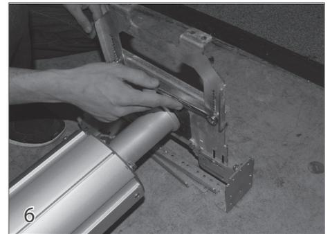
Install the mounting feet on the non motor end using the bolts (47) and lock washers (48) provided. The top of the pulley bracket on the non motor end should be flush with the top of the track.
