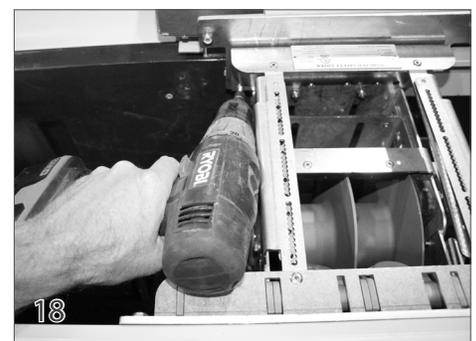
**Anchoring The Pulley Brackets**
