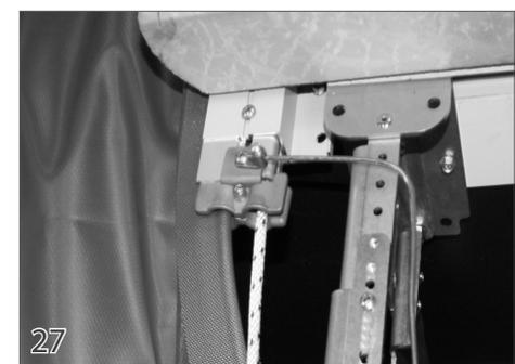
Run #8 copper bond wire (38) from the lug on each guide feed to the lugs on each end of the mechanism.
