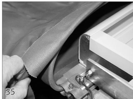
**Attaching The Cover & Bonding Wire**
