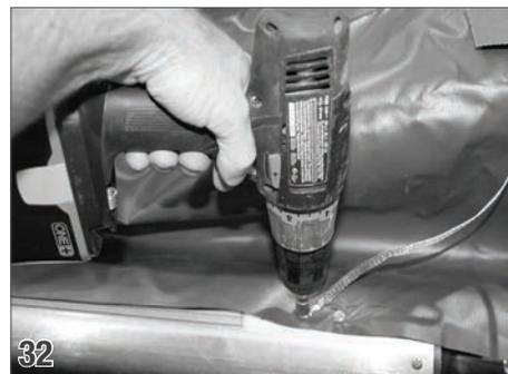
Lay the bond wire on top of the cover fabric. Secure it to the roll up tube using a tek screw (32). Distribute the slack of the cover evenly between each screw across the length of the tube. Secure the cover to the roll-up tube using tek screws (32) every 2-3ft. When attaching the cover to the tube, **do not use folds or pleats.**
