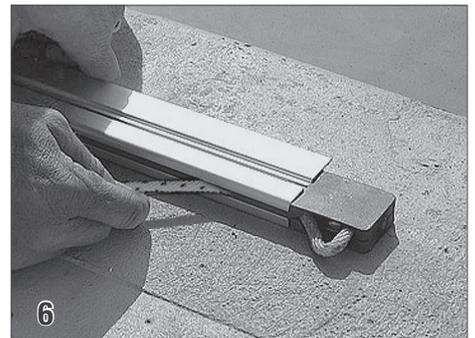
Now, feed the rope through the pulley assembly. Insert the pulley into the end of the guide.
