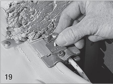
Place a guide feed over the end of the guide, place a bonding lug (25) on top of the guide feed. Insert a 10-32 x 1 3/4" screw (42) through the lug and guide feed.
