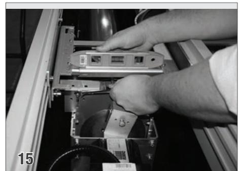
With the brackets in position, level the pulley brackets. Tighten the four nuts on the adjustable brackets.
