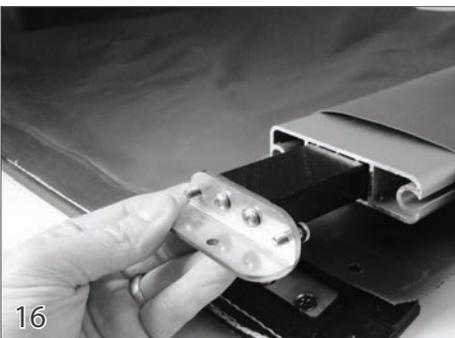
16 Insert the leading edge inserts into the leading edge tube.
