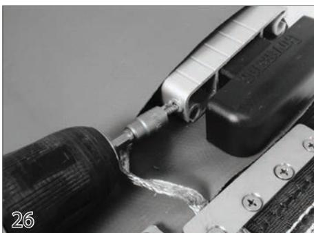
Attach the bonding wire to the leading edge bar using a self tapping screw (32).
