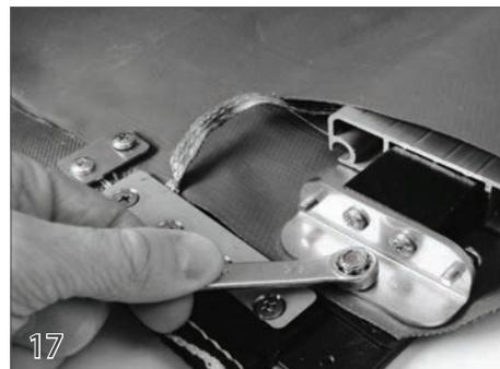
17 Attach the leading edge insert to the slider by inserting the a screw (41) from the bottom of the slider. The screw will go through a punched hole in the cover, then into the leading edge insert. Secure using a 10-32 Nylock Nut. (29)
