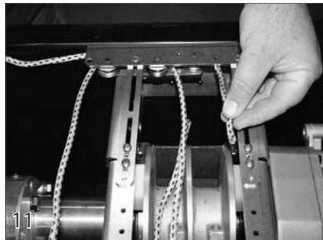
11 Feed the non-motor end rope behind the first and second and third horizontal pulleys.
