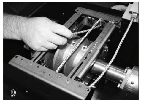
Pull the rope around the vertical pulley on the front wall of the housing.
