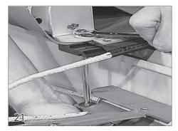
Secure the leading edge insert support bracket to the slider by placing the 10-32 x 1" screw up through the slider, through the hole in the front corner of the cover, and through the support bracket. Tighten completely using a 10-32 nylock nut, then back the nut off 1/2 turn.
