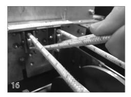
Insert the second rope in the same way into the other vertical pulley.
