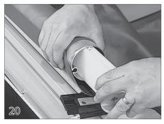
Place the nylon leading edge inserts into the ends of the leading edge tube. Make sure the inserts can slide freely inside the leading edge tube. If they don't, clean off any burrs that may be causing them to bind.
