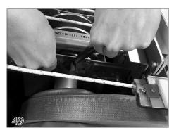
After adjusting the set screw, retighten the jamb nut while holding the set screw with an allen wrench. There's a corresponding brake on the opposite side of the rope reel. Adjust both brakes equally.
