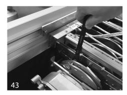
To adjust the torque limiter, use a 9/16" wrench to tighten the first tension bolts. It is important that the bolts are tightened equally.
