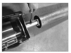
With the motor end turned upside down, attach the cone to the motor end of the mechanism using the 3/8" x 1-1/4" bolts (39) and lock washers (40) provided. Tighten these bolts with a 9/16" wrench.
