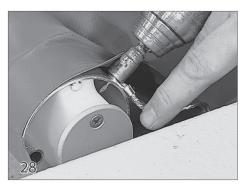
Connect the bonding wire that is attached to the front corner of the cover to the leading edge bar using a  $10 \times 1/2$ " tek screw (28). Be sure the screw doesn't interfere with the leading edge insert from moving freely inside the tube. Do this on both sides of the cover.
