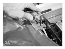
Use the allen wrench to tighten the screw that connects the two sections of guide feed together.
