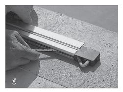
Feed the rope through the pulley (12) assembly. Insert the pulley with the rope onto the end of the track.
