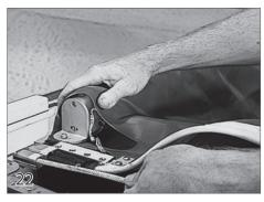
Pull the rope where it comes out of the track as you feed the slider and cover into the track. Keep pulling until the slider is in the track completely.
