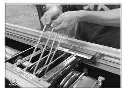
While holding the ropes over the mechanism, run the key switch in the cover position. As the excess rope is wrapped around the rope reel, make sure it goes on straight without getting crossed with each other.
