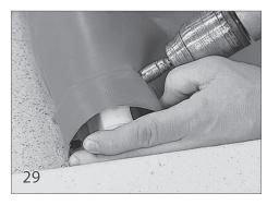
Position the fabric on the leading edge so it is in line with the leading edge support bracket. Secure with a  $10 \times 1/2$ " tek screw (28) on the back side of the leading edge tube. Be sure the screw does not interfere with the leading edge insert. Do this for both sides of the cover.
