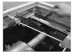
Loosen the bolts on the adjustable brackets on the non-motor end of the mechanism. Spread the pulley brackets outward against the walls of the cover box.
