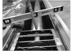
With the mechanism and tube assembled and set in place in the housing, check the roll-up tube for level. This is crucial to proper operation of the cover. Position a level across the housing. Measure from the roll-up tube to the bottom of the level on both the motor end and non-motor end of the mechanism. Adjust height of the non-motor end feet if needed to level the roll-up tube.
