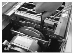
If further adjustment is needed, tighten the 4 bolts in equal increments 1/4 turn at a time.
