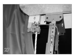
Run #8 copper bond wire (32) from the lug on each guide feed to the lugs on each end of the mechanism.
