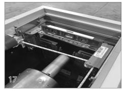
With the brackets on the non-motor end in position, place a small level across the brackets to make sure they are level. Tighten the nylock nuts on the adjustable brackets.
