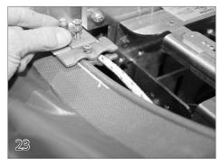
Use a 5/32" allen wrench to loosen the screw on top of the guide feed. Place the guide feed over the end of the track with the cover coming through one side and the rope through the other. Place a bonding lug (22) on a 10-32 X 1-3/4 screw (36) and insert the screw through the hole on top of the guide feed.
