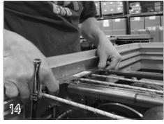
Raise the pulley brackets up so that the top of the bracket is even with the top of the encapsulation. This insures the ropes will be level.
