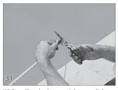
While pulling both ropes tight, use a lighter or torch to burn the rope in the location it will be cut. This will help them not fray after they have been cut. Cut the ropes so they are at least 8 ft long. In some cases you may only need to cut one rope. Use the lighter to re-burn the cut ends of the rope if needed.
