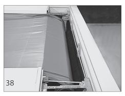
Run the key switch in the uncover position to roll the cover up on the roll-up tube. Check the cover to be sure it rolls up evenly. Run the cover 6-10 times to make sure it opens and closes evenly. The cover fabric installation is now complete.
