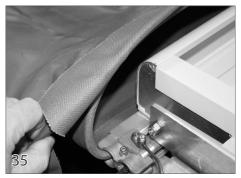
Attaching the Cover & Bonding Wire Make sure the webbing continues straight as it travels from the track to the roll-up tube. Attach the cover to the roll-up tube using tek screws (28). The first screw on each end of the tube needs to be 3 inches from the end of the tube. As the cover rolls up on the tube, the webbing will be rolling up over the cone.
