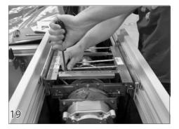
On the motor and non-motor side, use the half inch screws (24) and nylock nuts (26) provided and secure the cross braces together.
