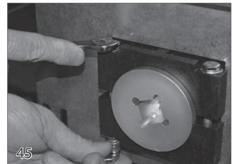
The roll up tube brake on the non motor end should be tight enough to prevent the cover from rolling off the tube faster than it is being pulled into the track. To adjust this brake, use two 7/16" wrenches and tightening or loosening the thru bolts in the brake block.
