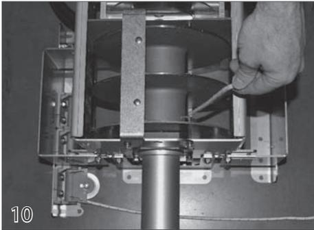
10 Direct this rope under the rope reel, over the rope containment bracket and out of the mechanism.
