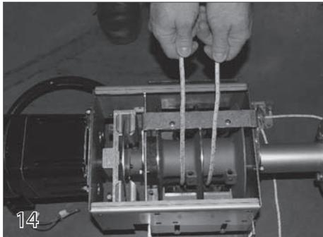
14 Pull the rope under the rope reel, over the rope containment bracket and out of the mechanism.
