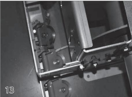
13 Bend a curve into the end of the wire and pull it back just until it is in the middle of the pulley. Now push the wire back until it comes out the side of the third pulley.
