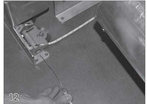
12 Insert the wire that is attached to the rope into the channel behind the first pulley. Continue to push the wire until it comes out of the channel behind the third pulley.
