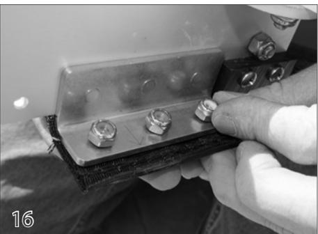
16 Attach the detachable rope tab to the three hole plate on the wheel assembly.
